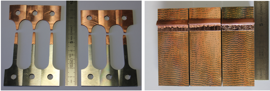
(a) Specimens of Plate 2, tested in tension, at 4.2 K (left) and RT (right). (b) Specimens of Plate 5, tested in shear, in longitudinal direction (LD).
