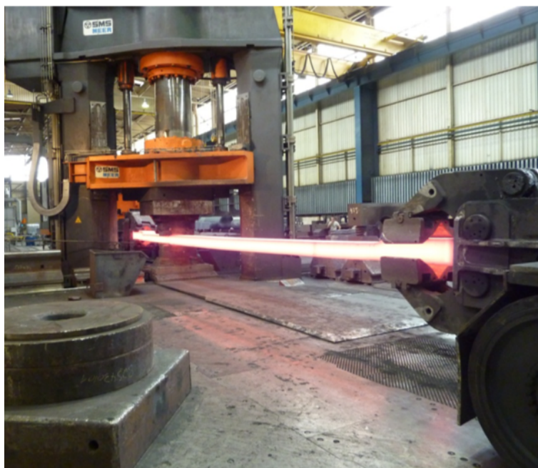
Figure 2.1: Photograph showing the 15 m tie plate forging from a single piece. Note that this image is taken during an intermediate forging step, is indicative, and thus not contain the full length of the end-piece. The image illustrates the manipulation of the piece on the one end, and the challenges to maintain dimensions and straightness [Degitz, 2013].
