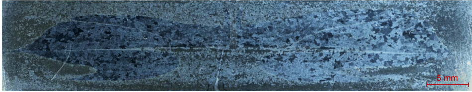
(b) Image of the conductor cross-section (without cable), showing the transition from Al-0.1wt.%Ni to 5N-Al.
